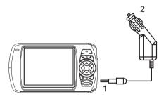
When the battery is in a low voltage, you can recharge it in the car:
